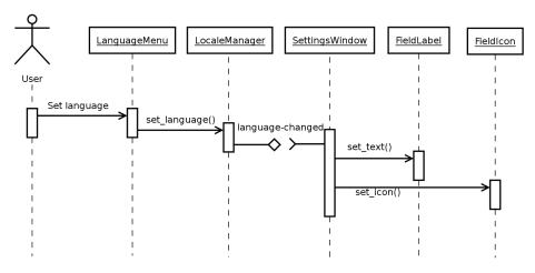
LocaleManager in the diagram would be a singleton that stores the current locale and notifies interested parties when it changes. The current locale would be changed by UI elements such as a combo-box in the settings panel, a menu option, etc.
